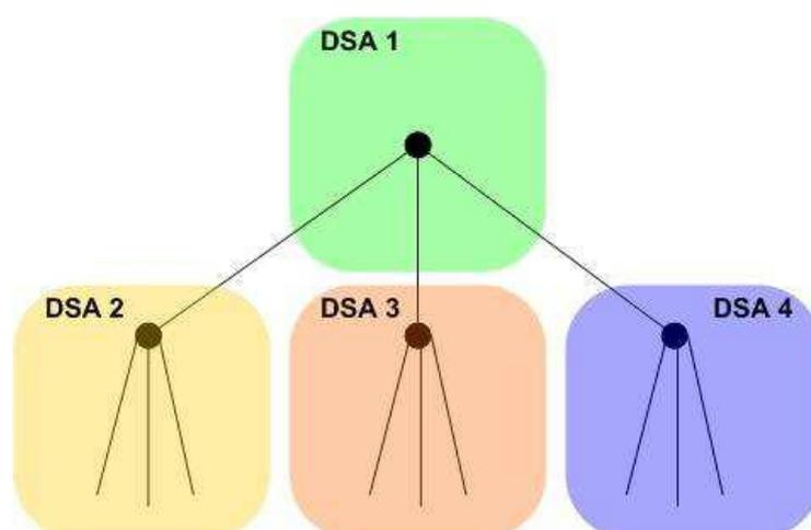
There is no limit on the number of different servers that are present within the distributed environment and each server can work cooperatively to service a client's request. DSA to DSA communications is achieved through the support of DSP – The Directory System Protocol, which allows a DSA to interact with other DSA's in order to service a request on behalf of the client.
