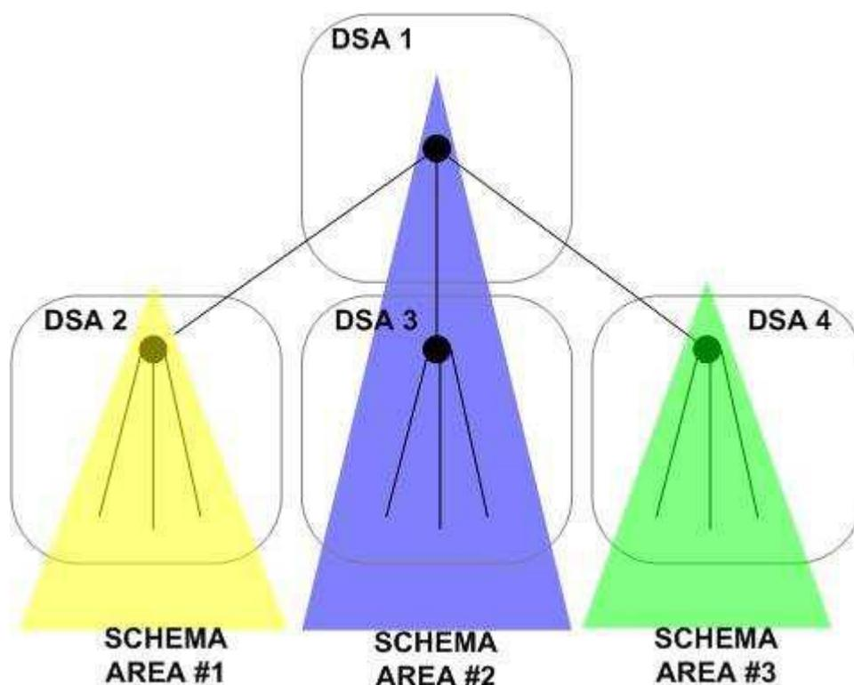
The ability to maintain schema in the DIT results in the efficient management of the schema in a distributed environment. In the image above, DSA #3 doesn't need to define new schema, since the distributed data model allows it to automatically retrieve it from its parent, DSA #1.
